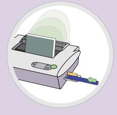
**STEP 2**: Insert binding strip into feeder.
